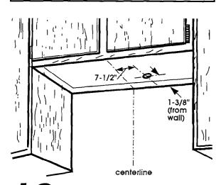
7-1/2" from the right of the centerline on the underside of the cabinet. Mark the point on this line that is 1-3/8" from back wall. Drill a 1-1/4" diameter hole through the cabinet at this point.
